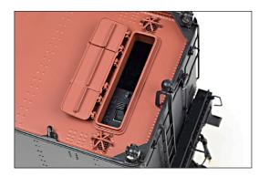
The image to the right illustrates the arrangement of the sound controls as though looking through the cistern hatch facing to the front of the locomotive. The controls should be adjusted using a small plastic screwdriver to prevent shorting the circuit board should you touch it during the adjustment.
