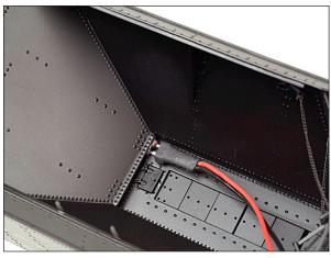
The photograph to the left shows the sound/ control system on/off switch under the cistern hatch. The sound controls are accessed under the hatch to the right of the switch.
